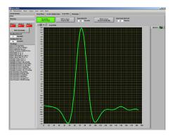
The location of the peak on the X-axis confirms the identity of water. The y-axis is related to the partial pressure of water and therefore the concentration. The system is equipped with AuroraView software, which enables users to capture the absorption spectrum and export it to other application programs such as Excel<sup>TM</sup>.
