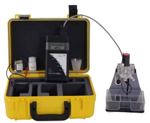
The PDV6000*ultra* has been upgraded to allow much improved stand-alone operation and an indication of blank and standard run performance. A larger screen allows simple voltammograms to be shown. The USB connector replaces the serial port. The upgraded product has a battery life indicator and can be run either on  $4 \times 1.5V$ AA batteries, or from the mains using the standard 8 - 12V DC transformer.
