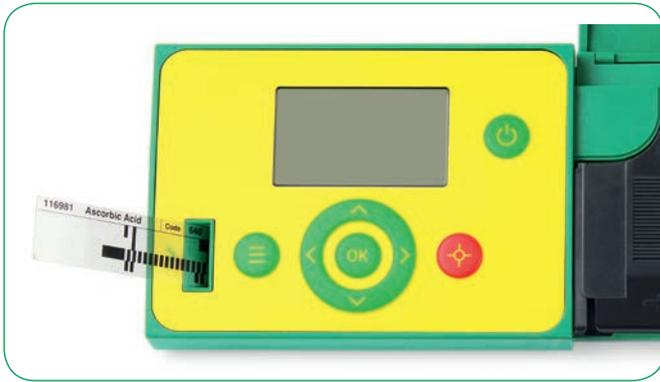
For every test condition, each batch of test strips is calibrated and equipped with a barcode for accurate and reproducible results. Obtain consistent results quickly with an average accuracy within  $\pm 10\%$  in the middle of the measuring range.
