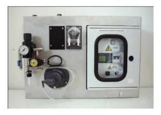
For waste water or other dirty samples application a self cleaning filtration unit can be installed close to the analyzer. Thanks to the integrated PLC, the filtration unit runs periodically a self cleaning cycle, using compressed air generated externally or even internally (as option). One filtration unit can be used to supply a clean water sample up to 10 analyzers.
