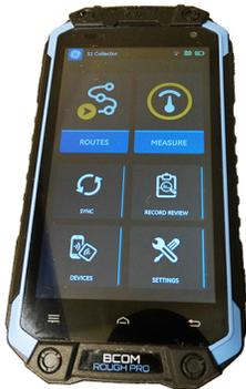
The data collector uses Bluetooth to communicate with the industrial handheld which is also rated for hazardous environments. The S1 Collector app exchanges data with System 1 Evolution via Wi-Fi or a cellular network.
